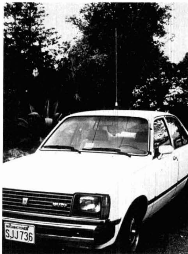
fig. 1. Mag-mount whip antenna after modification and installation.
